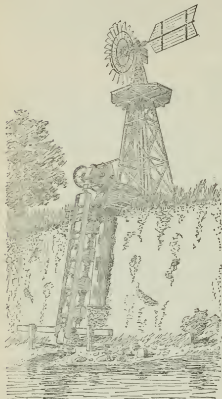
FIG. 33.—Bucket pump operated by windmill.
