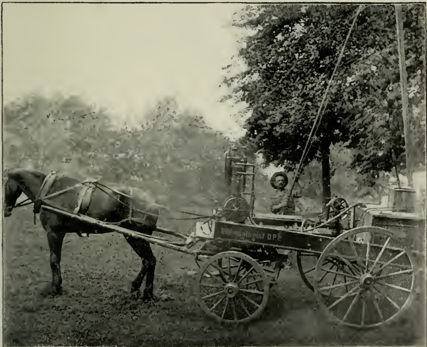
FIG. 2.—VIEW (FROM OPPOSITE SIDE) OF STEAM SPRAYING APPARATUS USED BY THE DEPARTMENT OF PUBLIC PARKS OF NEW YORK CITY, IN OPERATION.
