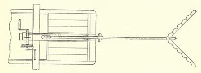
Fig. 100.—Hand-power Machine for fixing to Boats or Punts, which may be rowed by oars or towed from the bank by ropes. The cutting is performed by the V-shaped scolloped saws suspended from an oscillating hinged arm. A similar V-shaped weed-cutter on a long handle is useful for hand work from the bank, boat or punt. (Saunderson, Bedford.)
